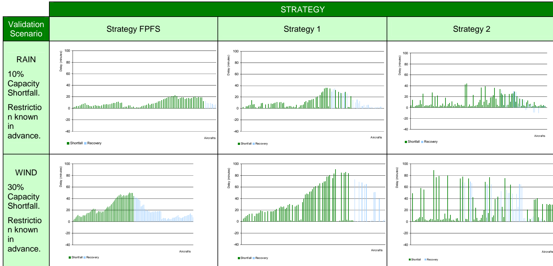
Figure 27: Delay distribution when applying a DCB Queue process to the same traffic sample for Validation Scenarios Rain and Wind and the three strategies.
